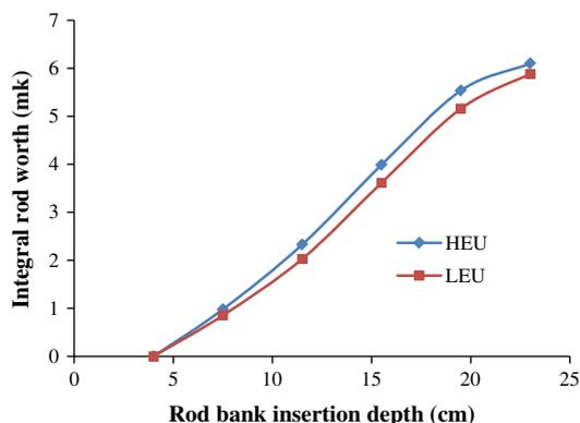
**Fig. 4.** Integral worth of ASCRs versus depth from the bottom of inner channels for HEU and LEU cores.
