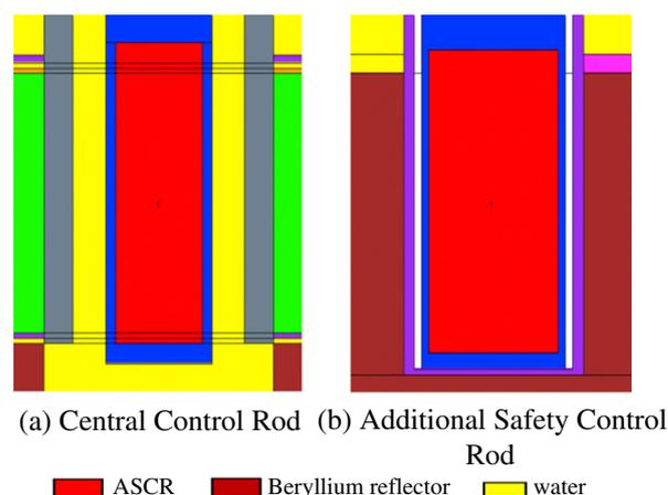
Fig. 2. MCNP geometric representation of central and ASCRs.
