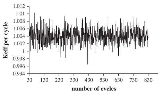
Fig. 3. Power iteration for Monte Carlo criticality calculation of the mean value of  $k_{eff}$ .
